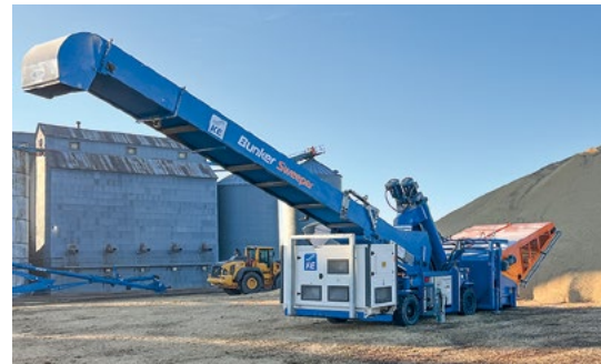
KE BunkerSweeper750 with onboard generator
