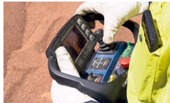
Wireless remote with camera feed from discharge chute to screen
