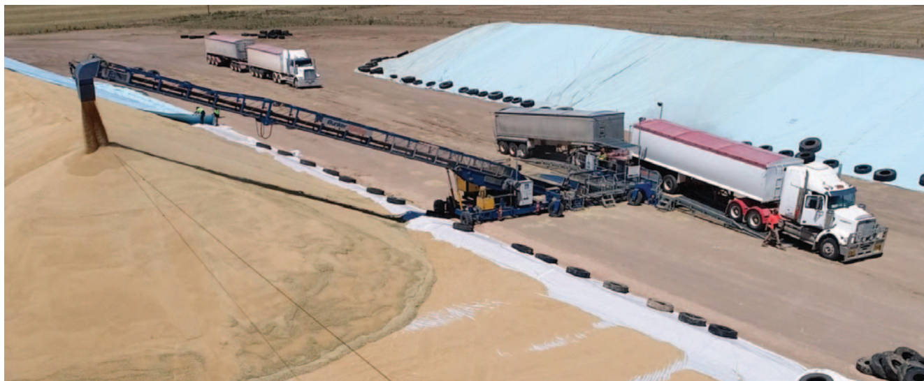
KE's new UBA (under belly auger) hopper conveyor unloading Canola (rapeseed) on a BunkerStacker3000 Roo machine (and above).
