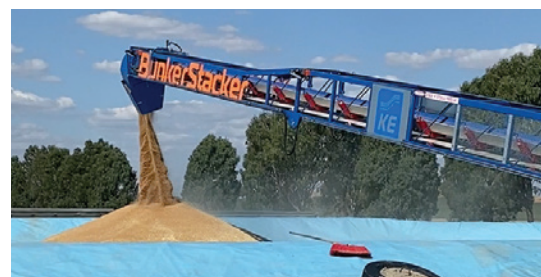
Multi-directional discharge chute to make trimming the bunker or grain pile easy
