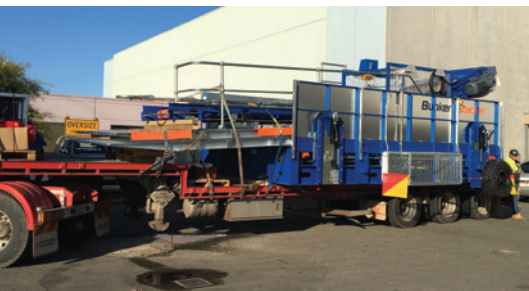
The BunkerStacker 3000 can be moved between sites on two semi-trailers
