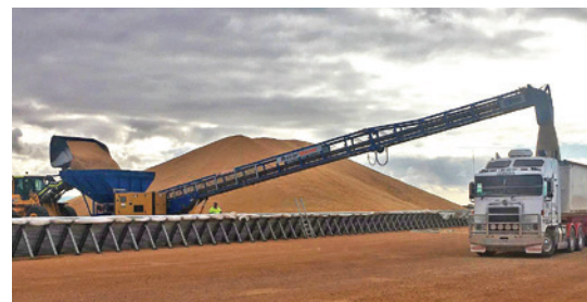
Outloading via BunkerStacker 3000 fitted with surge hopper
