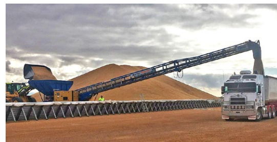
Out loading via BunkerStacker 3750 fitted with surge hopper
