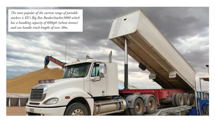
BunkerStacker range of portable equipment is its capacity to be used in reclaim mode with the stacker component fitted with a surge hopper which is generally fed by a front-end loader (FEL) for easy out loading from the product stack to trucks.
