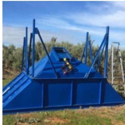
**2.** Remove the first two 20mm stanchion leg bolts closest to the square side of the hopper.
