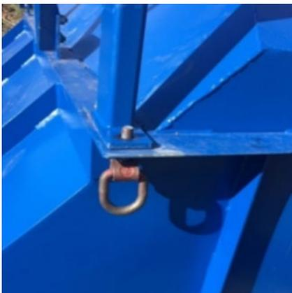
**3.** Using 2 x M20 RUD lifts, attach them to the hopper as per photo instructions and as per manufacturers recommendations (4 better lifting guide).
