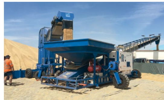
Outloading via BunkerStacker
