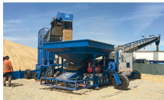
Outloading via BunkerStacker
