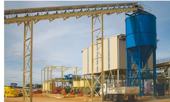
Belt Conveyor on trestles for loading of mineral sands – Mindarie, South Australia
